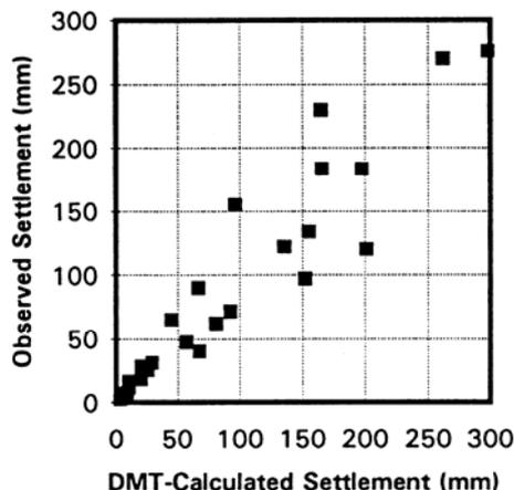
Fig. 4. Observed vs DMT-calculated settlements (Hayes 1990)
