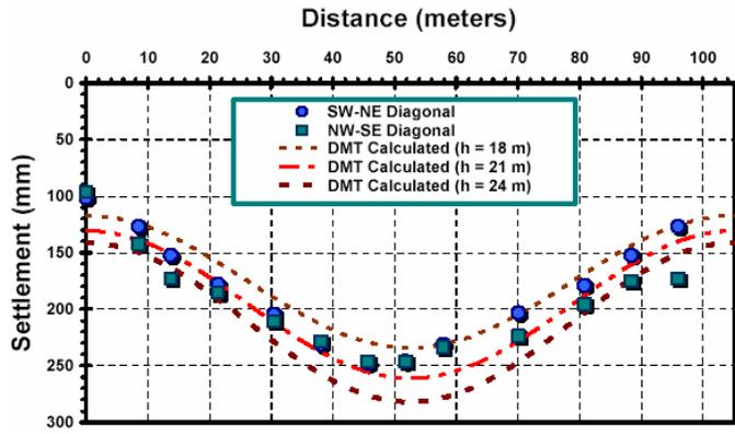
Fig. 7. Measured vs DMT-calculated settlement profiles along the diagonal axes of the mat foundation of a 13-story dormitory building in Atlanta, Georgia (Mayne 2005)
