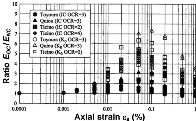
Fig. 9. Effect of OCR on *secant* Young's modulus from triaxial tests on NC and OC sand specimens (Yamashita et al. 2000)
