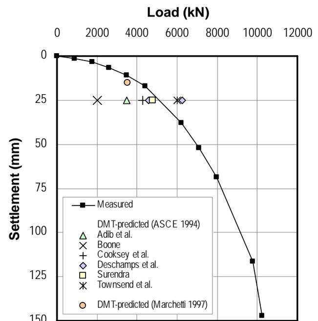
Fig. 5. ASCE Settlement '94 Spread Footing Prediction Symposium. Measured load-settlement curve for Footing 1 (3x3 m) vs values of load  $Q_{25}$  predicted by DMT by various Authors (ASCE 1994) and additional prediction by Marchetti (1997)
